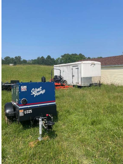
Photograph No. 4 Silent pump generator.
