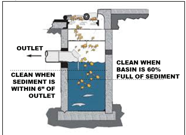
Remove sediment from a catch basin if it fills 60% of the sump or comes within 6" of a pipe.
