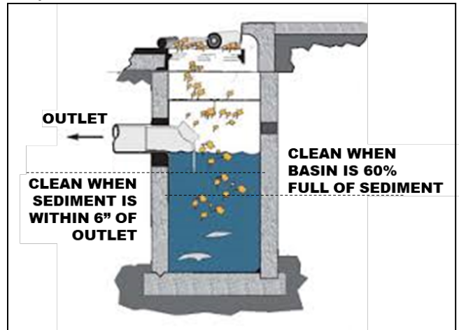
Remove sediment from a catch basin if it fills 60% of the sump or comes within 6" of a pipe.
